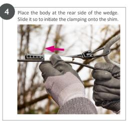
Secure the cable by pulling the clamp's body towards the span side while maintaining the bail.
