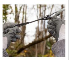
Place the flat cable into the clamp's body.
